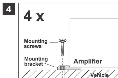
Then uphold the amplifier to the chosen position and fix the screws through the holes of the mounting brackets into the drilled screwholes. Ensure that the mounted amplifier is fixed tight and not get loosen.
